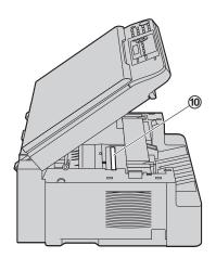
7 Install the drum and toner unit (1) by holding the tabs.
